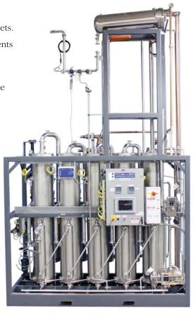
As the pure steam is condensed in the shell side of the subsequent evaporator, the resulting WFI flows through feedwater preheating devices and to the WFI condenser for subcooling to the required product temperature. Only pure steam discharged from the last effect of the still is condensed in the product condenser. The final product as well as the feedwater supplied to the still is measured for conductivity to ensure compliance with specifications.
