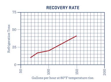
$<sup>^{1}\</sup> Refrigeration\ tonnage\ capacities\ are\ 30^{\circ}F\ evaporator\ ton\ loads,\ not\ total\ heat\ of\ rejection\ tons.\ Pressure\ drop\ through\ a\ Fre-Heater\ refrigeration$  $circuit\ will\ be\ approximately\ 15\ psi\ at\ the\ maximum\ tonnage\ application.\ Pressure\ drop\ at\ the\ mid-range\ of\ tonnage\ application\ will\ be\ about\ 5$ to~7 psi.~The~best~over all~refrigeration/heat~recovery~system~efficiency~is~usually~obtained~at~or~below~the~mid-range~tonnage~application.
